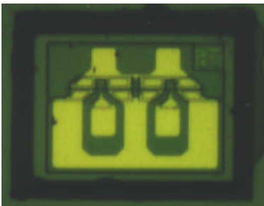
Fig. 3: (a) Top view of GaAs PHEMT chip mounted in a Si Substrate.
